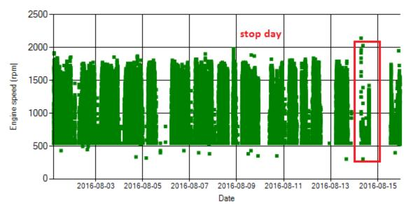
Figure 9- Engine speed diagram for calculating CPK's working days
