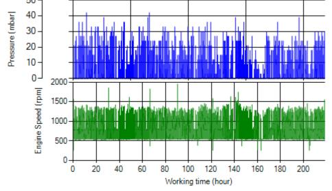
Figure 12- P, N distribution vs. working hours
