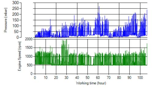
Figure 14- P, N distribution vs. working hours
