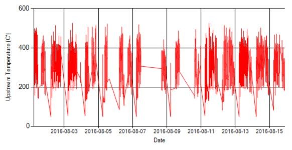
Figure 6- Temperature distribution over the period
