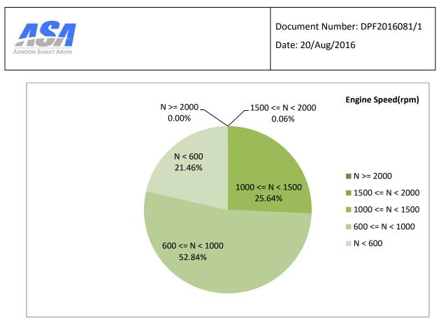
Figure 3- Engine speed distribution over the working hours
