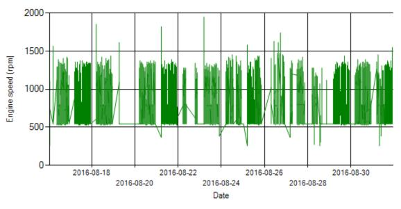
Figure 8- Engine speed distribution over the period
