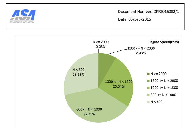
Figure 3- Engine speed distribution over the working hours
