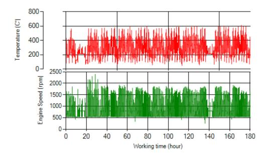
Figure 14- T, N distribution vs. working hours
