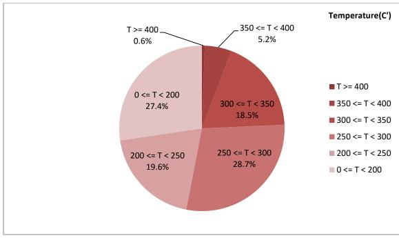
*Figure 2-Temperature distribution over the working hours*
